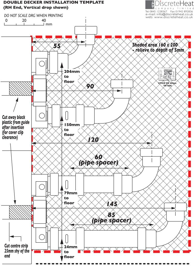
Vertical pipe drops shown. Reverse for through-floor feed & returns (see P2)
