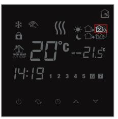
Press  $\bigcirc$  again to enter into  $\textcircled{}_{\bullet}$  3rd time period/ temperature setting and repeat as above.
