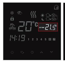
Press , again and the target temp starts flashing (default: 22°C), press , or  $\checkmark$  to set target temp.
