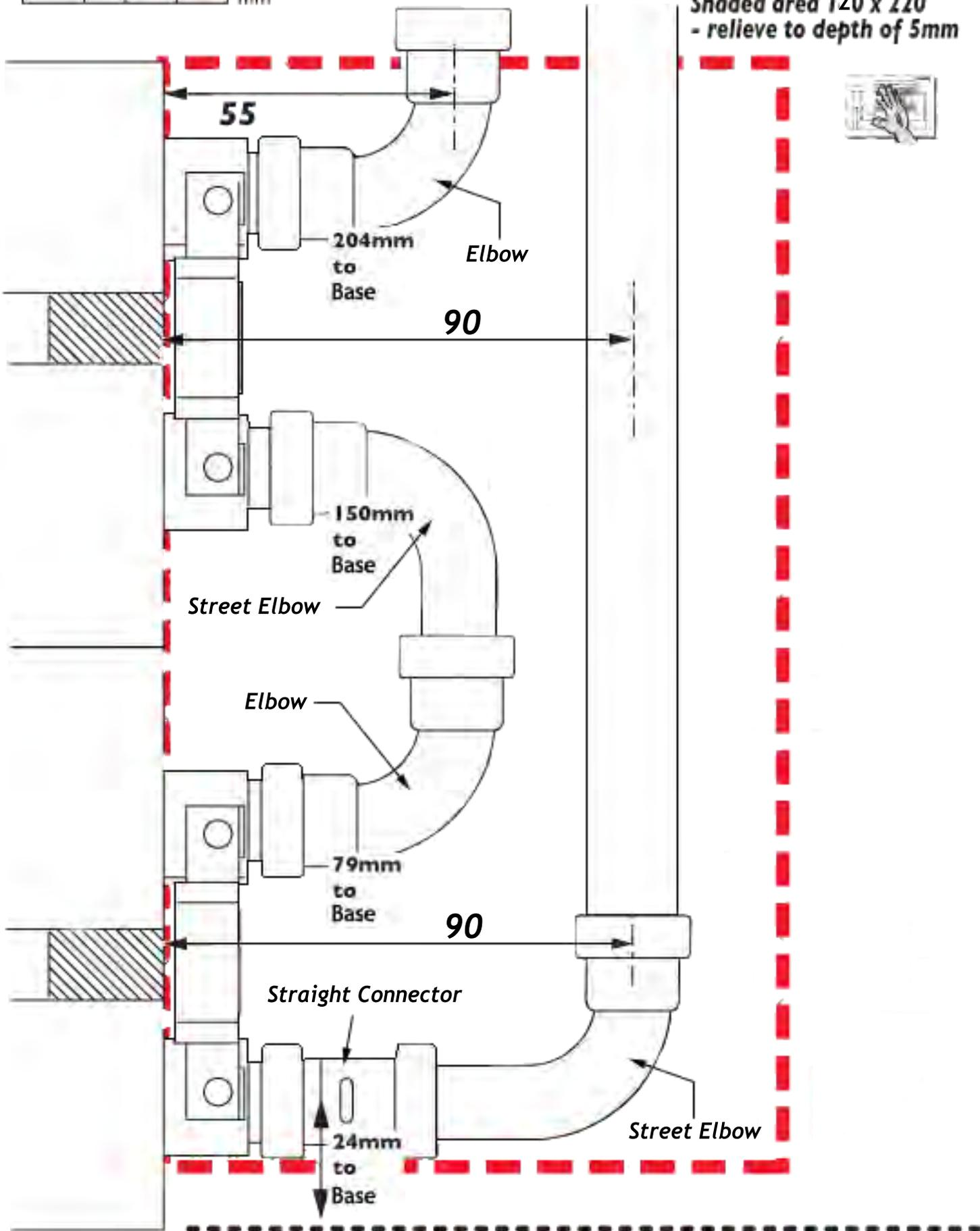
Vertical pipe drops shown. Reverse for through-floor feed & returns (see P2)
