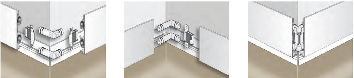
TIP: If any of the mounting rails interfere with the elbows or return manifold, then the mounting rail can be nibbled away using pincers.
