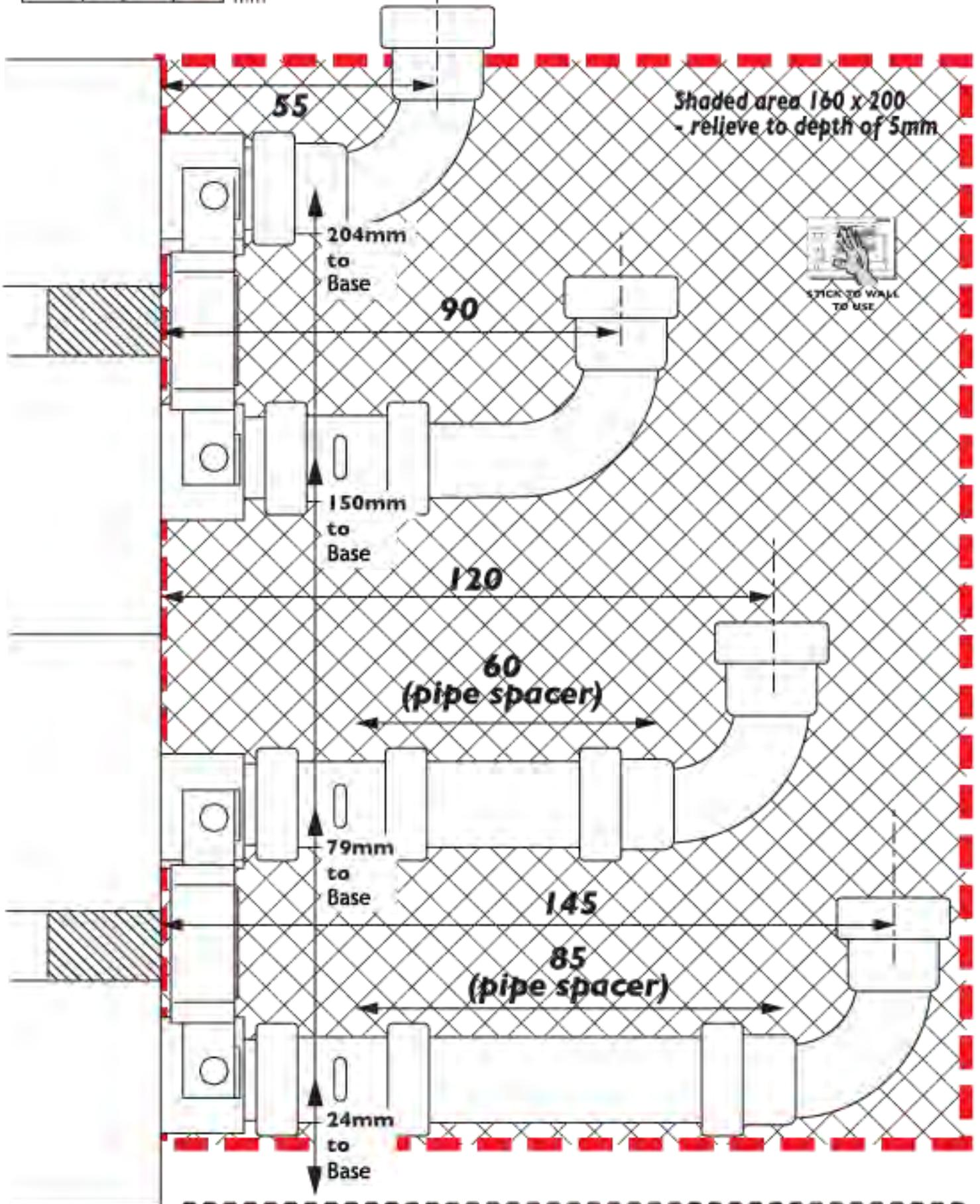
Vertical pipe drops shown. Reverse for through-floor feed & returns (see P2)
