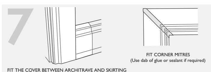
If required the assembly can be caulked or sealed for a perfect finish
